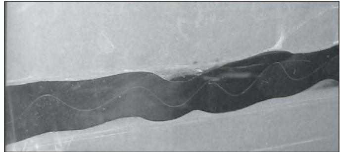
*Failure mode – exceeding the adhesive working time*
